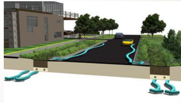
Channeling Storm water
